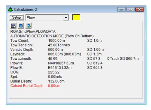
From this window, you can monitor some of the input data as well as the layback calculation, if it's used. This Calculation window also provides a shortcut to the Configure Plow dialog box by clicking the button.
