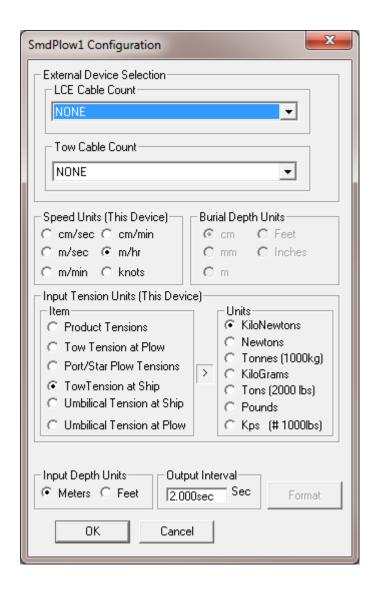
From the dropdown list boxes select the data source (device) for the LCE telephone cable count data and the Tow cable count data. Also select the appropriate Input Speed Units as well as the Input Tension Items and their associated Units. Specify whether the Input Depth Units are to be meters or feet.
